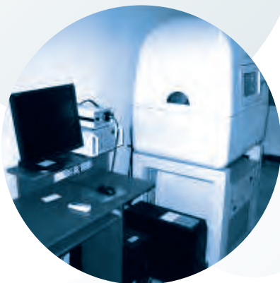
Hysitron TriboIndenter TI-900 for nanomechanical characterization
